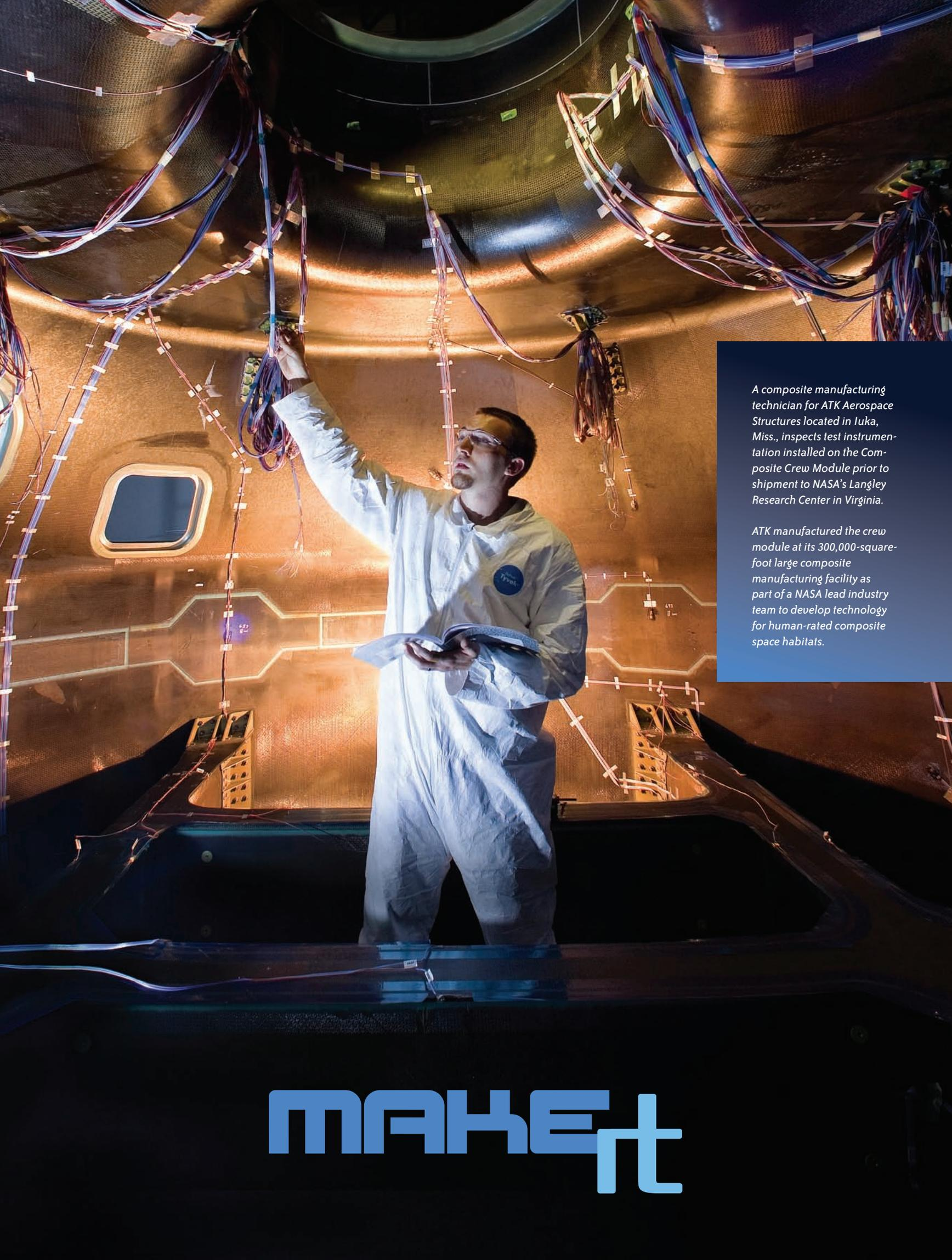
*A composite manufacturing technician for ATK Aerospace Structures located in Iuka, Miss., inspects test instrumentation installed on the Composite Crew Module prior to shipment to NASA's Langley Research Center in Virginia.*
